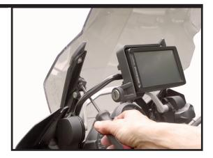
2 To install the **Slipscreen**, position it to engage the mounting tabs on the bike where shown, and align the two mounting holes.
